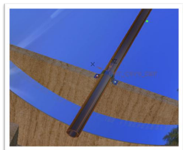
Fig -2.4: Absorber tube Strip Placement and Mounting
