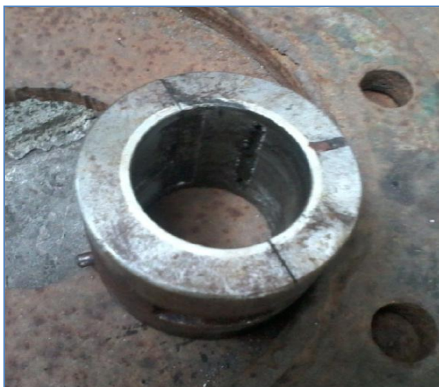
Figure No. 3.1 Bearing Failure in boiler feed pump
