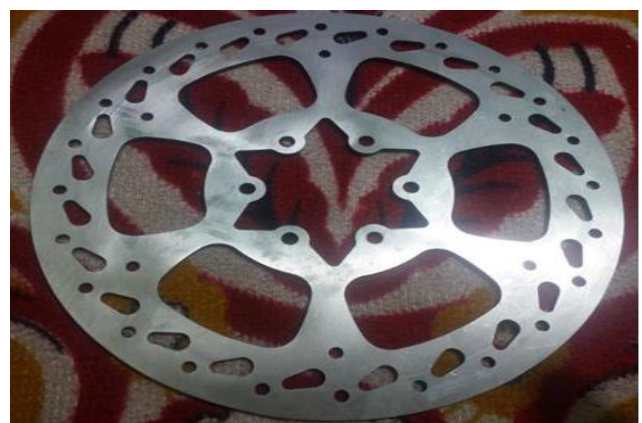
Figure 5.2.2: Disc-2 specimen after experimental test
