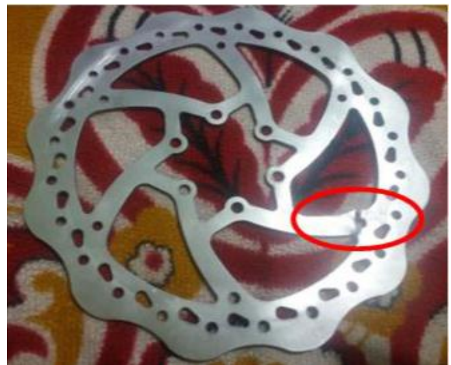
Figure 5.2.1: Baseline (Disc-1) specimen after experimental test
