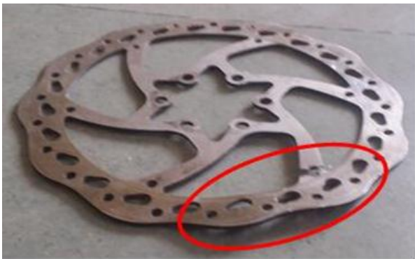
Figure 2.1: Bent and cracked disc
