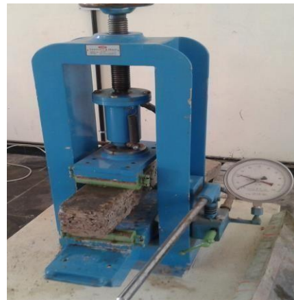
FIG.1: FLEXURAL TEST ON BEAM
