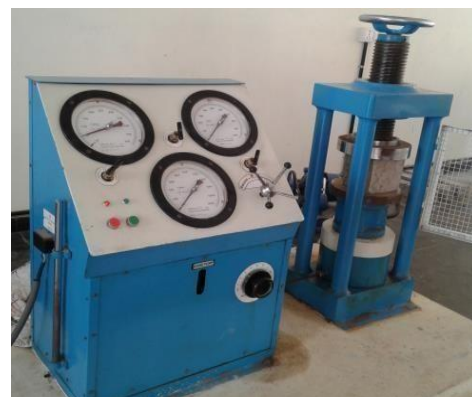
FIG.2: COMPRESSION TEST ON CUBE
