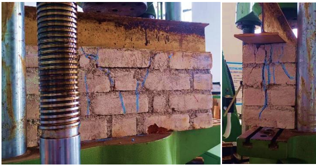
Fig -8: Failure of wall panels
