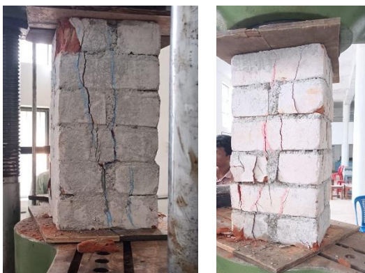
Fig -9: Failure of masonry prisms
