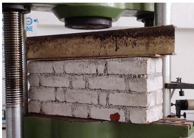
Fig -7: Testing setup of wall panels
