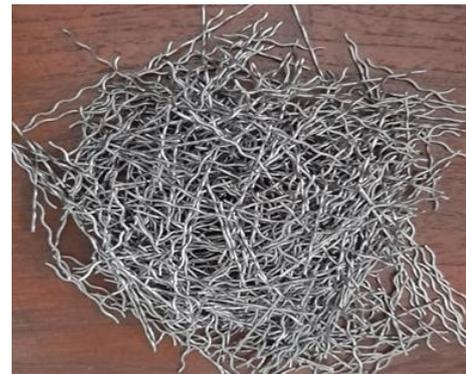
Fig -2: Steel fibres
