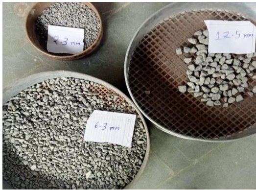
Figure 1.2 shows the sieving of FA
