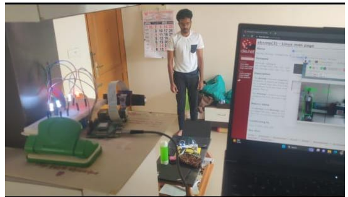
Fig-10: Person is identified in the sector and data is transferred to the NodeMCU
