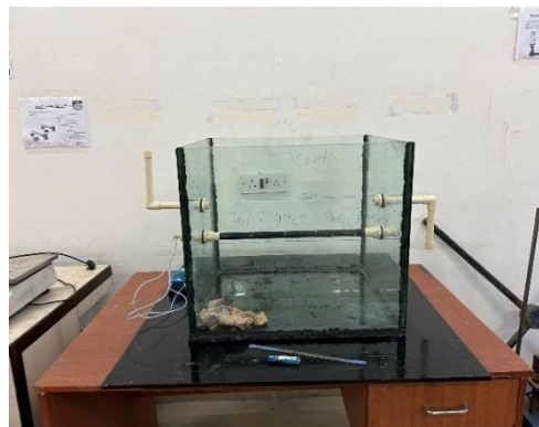
Fig 8: Assembled Prototype Model for phytorid Bed
