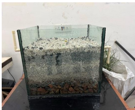
Fig 9: Phytorid Bed with Different Layers of Aggregate
