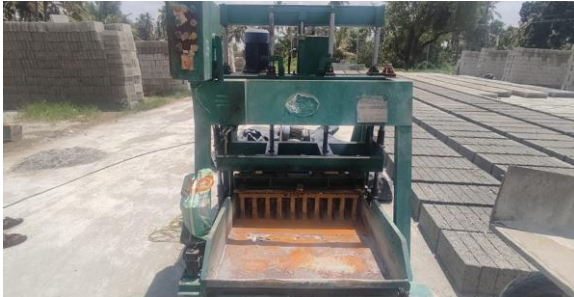
Fig 1 Punching Machine used to prepare blocks.
