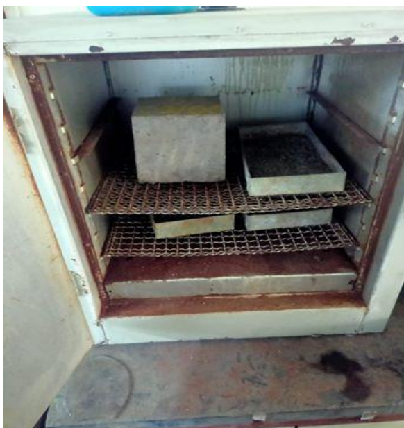
Fig -5: Oven drying of concrete cube
