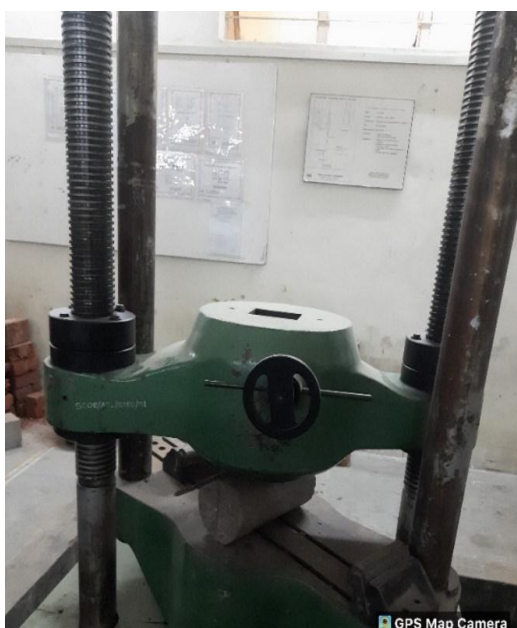
Fig -3: Split tensile strength testing
