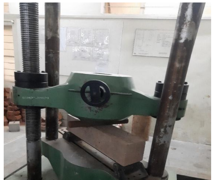
Fig -4: Flexural strength testing
