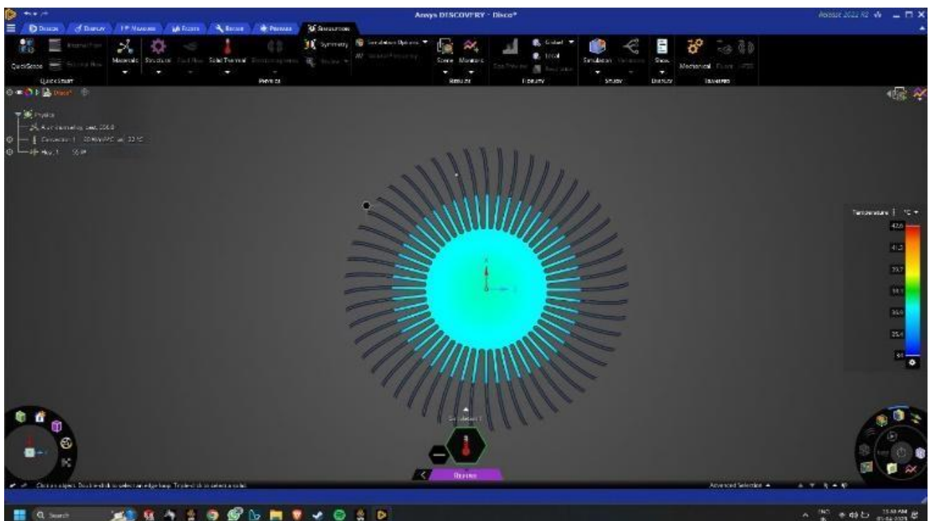
Fig. 6: The temperature contour of heat Sink in top view
