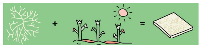
(Fig 2 Mycelium composite material manufacture process)
