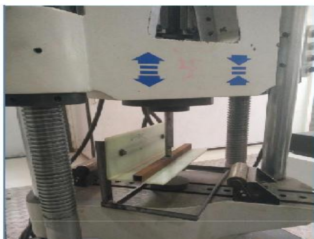
Fig.5.1:- Compression loading of GFRP bracket
