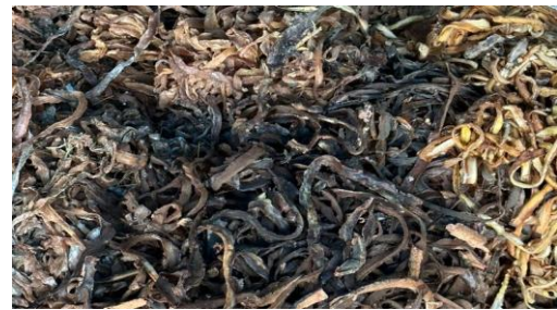
Fig-4: Natural rubber crumps
