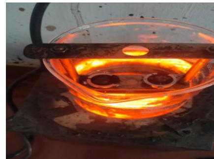
Fig-7: Softening point test in normal water
