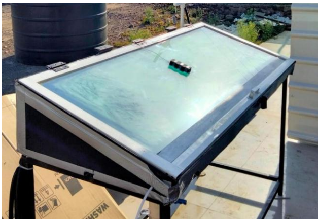
Fig -3: Fabricated Solar Still
