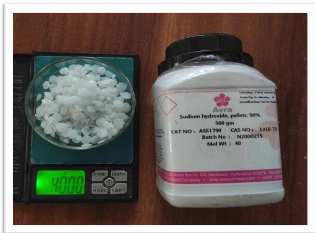
Fig 1: Weighing of NaOH Pellets
