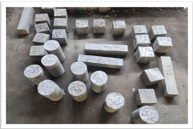
Fig 12: Chemically Treated Coir Fiber Reinforced Concrete are Unmoulded
