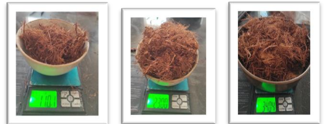
Fig 9: Weight of Treated Coir Fiber For 3 Different Mix Proportion
