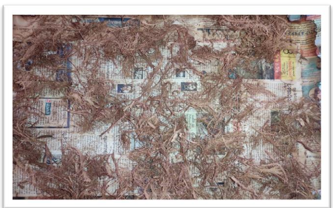
Fig 8: Treated Coir Fiber in Dry Condition After 24 Hours
