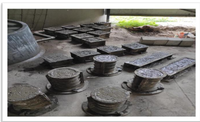
Fig 11: Chemically Treated Coir Fiber Reinforced Concrete are Moulded
