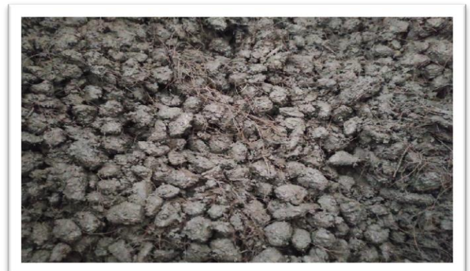
Fig 10: Treated Coir Fiber Mixed with Concrete
