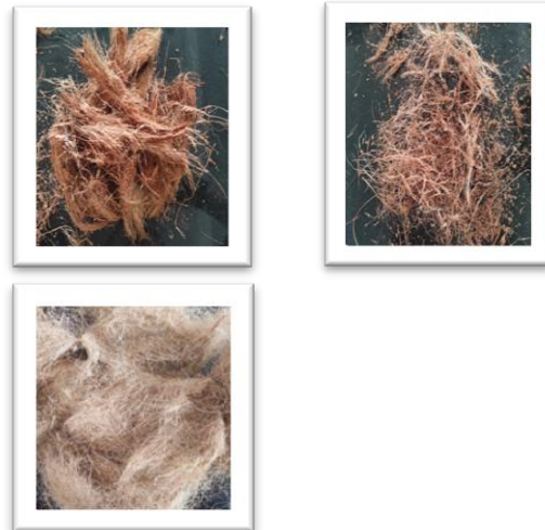
Fig 4: Extraction of Coir Fiber From Matured Coconut Husks
