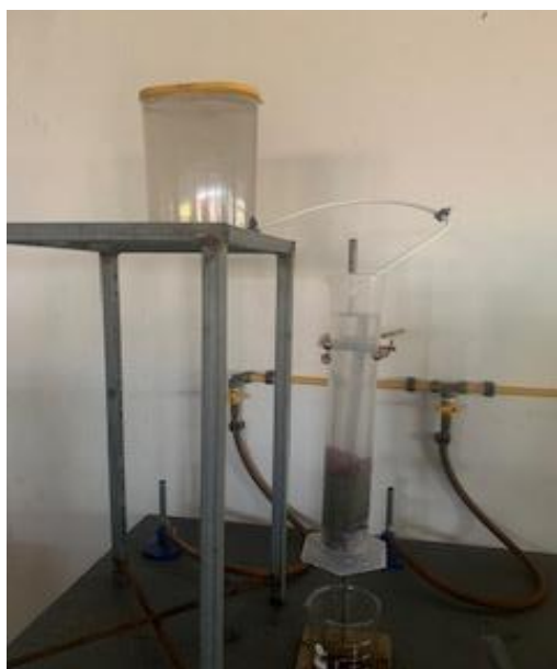
Fig -2: Column setup
