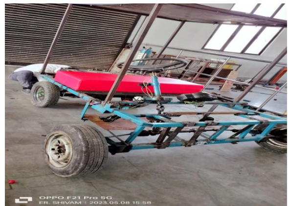
Figure 12- Complete fabricated car model of self charging electric car
