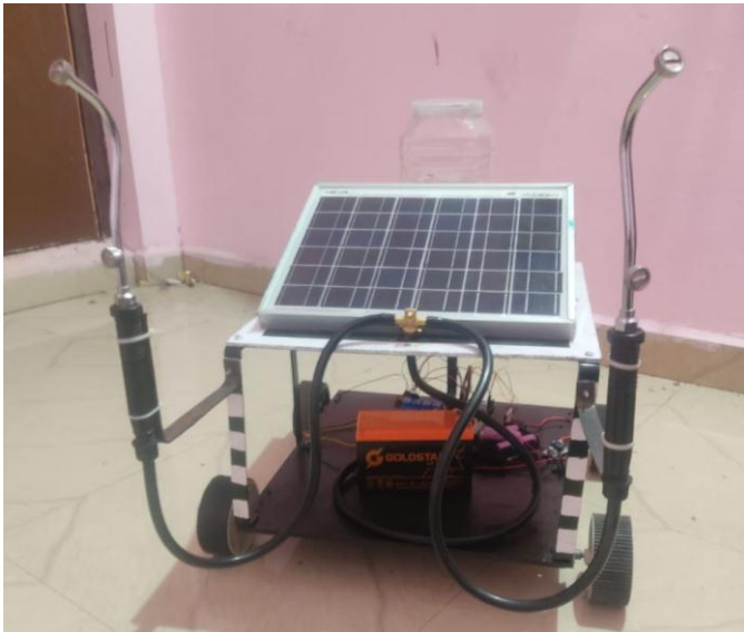
Figure 19. Physical look and end result of our designed Pesticide sprayer Robot (SprayRo)
