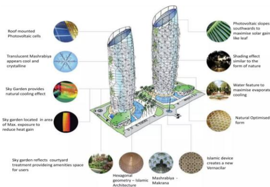
Figure – 3: Al-Bahr Towers Structure Description
