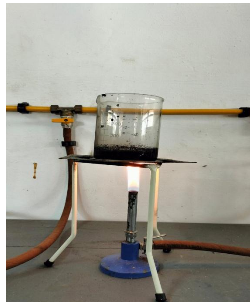
Fig-2: Activation of Saw dust ash
