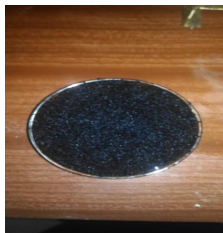
Fig-3: Saw dust activated carbon
