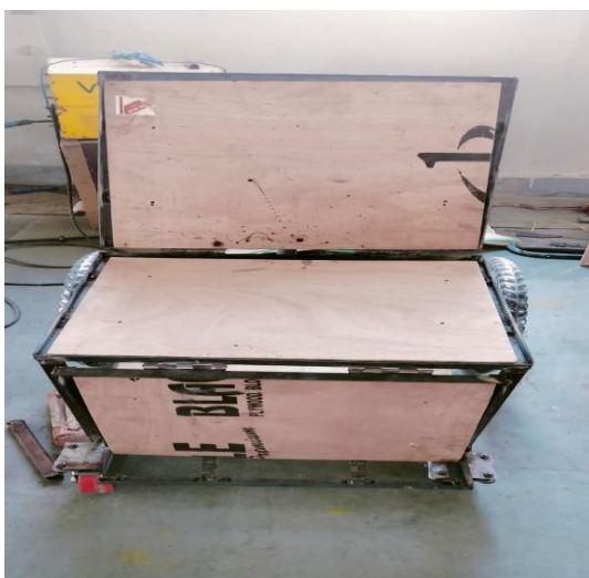
Figure 3: Complete base structure
