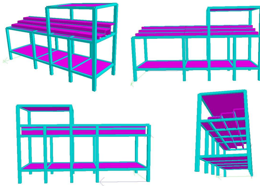
Figure 5. Concrete Tribune Structure Modeling with Staad Pro V8i Software
