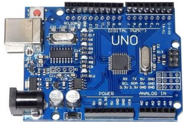
Fig-2: Arduino Uno board (ATmega328p)
