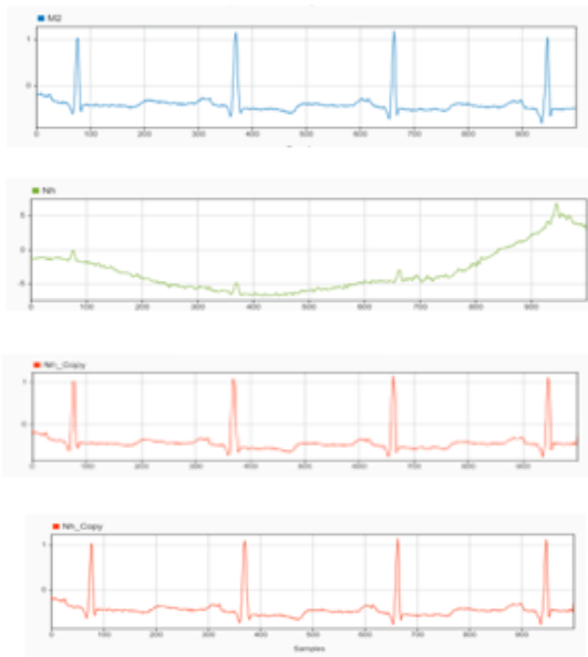
Chart -1: ECG, Noisy and De-noised signal (a) Healthy ECG signal, (b) ECG signal corrupted with BLW noise, (c) De-noised by LPF, (d) Filtered signal smoothed by Moving-mean method
