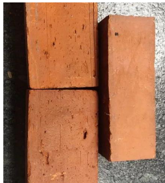
Figure 11:- Finishing of Conventional 2nd Class Brick
