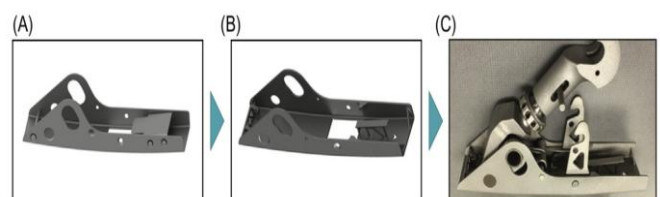
Fig.13: AM component consolidation of a jet engine cowl latch.
