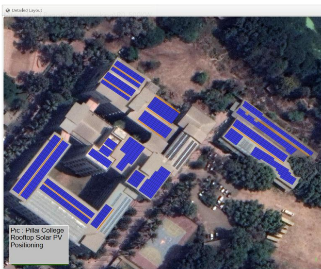
Figure: Rooftop Solar PV (500 kWp) Location Layout
