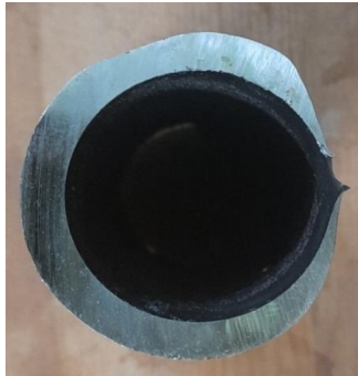
Figure 3.1 (c): Cross section at the failed region of RH tube.
