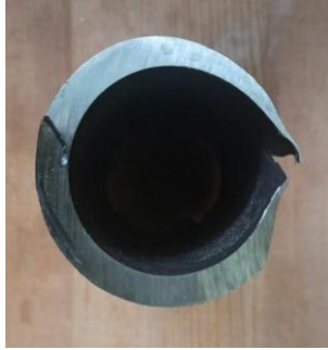
Figure 3.1 (b): Cross section at the failed region of Economizer tube.
