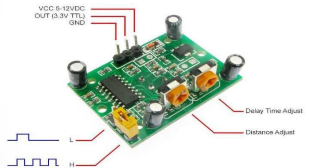
Fig -4: Pin layout of the PIR (Passive Infrared) sensor
