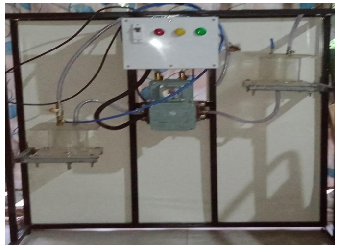
Fig.3. Actual model of Buchholz relay testing kit.
