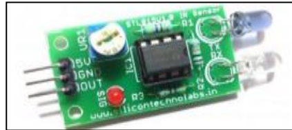
Fig 5 IR Proximity Sensor
