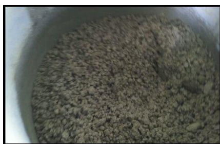
Fig.9. Fresh Geopolymer Concrete mix
