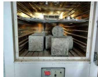
Fig.10. Oven curing of Geopolymer Concrete specimens
