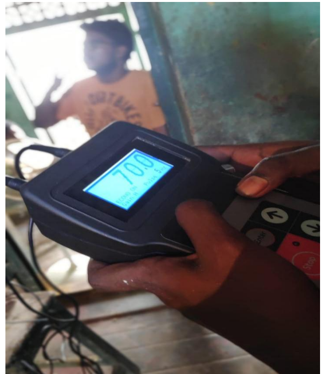
Figure 5.4: Ultrasonic pulse velocity test
