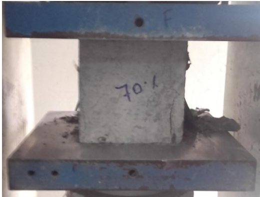
Compressive strength test
