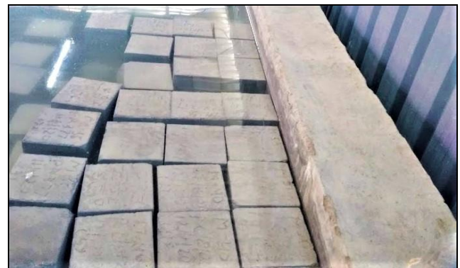
Fig -1: Curing Concrete Cube
