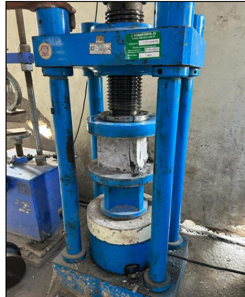
Fig -5: Cube under compressive testing machine
