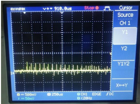
Fig.10 Power Line Receiver: pulses received from transmitter
