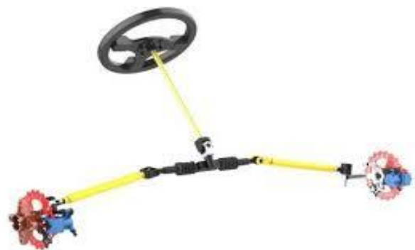
Figure 5: Assembly of the steering system
