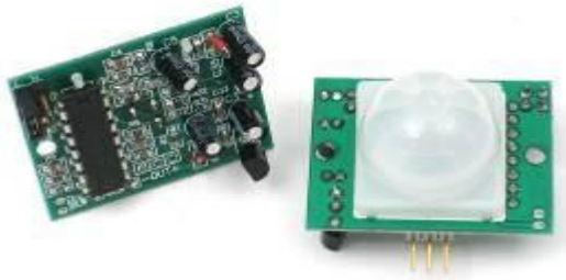
Fig -2: PIR Motion Sensor
