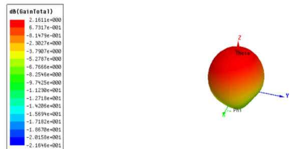
Fig-15: 3D Polar plot for gain of 1*1 rectangular patch without slots
