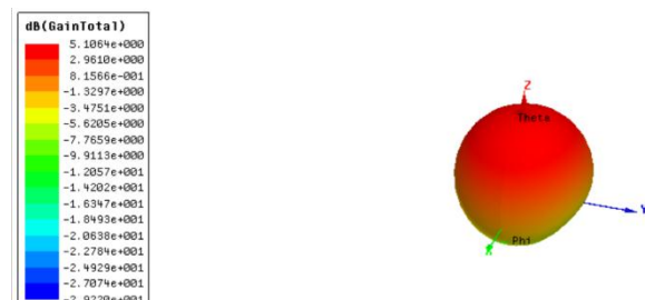
Fig-16: 3D Polar plot for gain of 1*1 rectangular patch with slots
