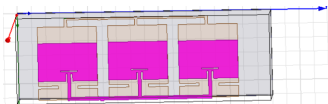
Fig-14: Modified 1*3 Rectangular Patch with Slots
