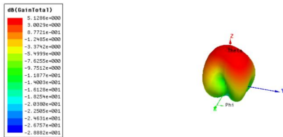
Fig18: 3D Polar plot for gain of 1*3 rectangular patch without slots
