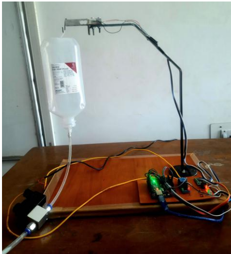
Fig 3 Here IV Bag fluid level is critically low so RED color LED is HIGH and the RELAY MODULE is ON to switch on the solenoid valve to stop the fluid flow
