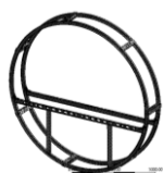
Fig 2- The meshed model of the Floor beam.
