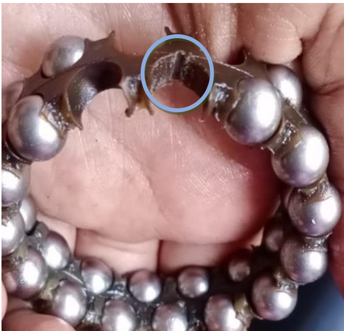
Fig -8: Cage defect
