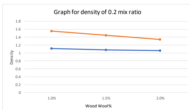
Graph 1 Density with mix ratio 0.2 and wood of varying %
