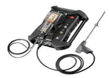
Testo 350 is a portable emission analyser, wherein we get the digital readings of amount of each gas coming out from the exhaust.
