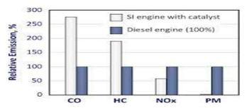
It can be observed from the above graph that, the NOx produced by diesel engines are way too higher than those produced by petrol engines, reason being NOx are formed at very high temperatures of order more than  $1100^{\circ}$ C. Whereas in a diesel engine the combustion temperature is around  $1100^{\circ}$ C, hence the amount of NOx formed by diesel engines is greater. Thus controlling NOx emissions from diesel engines is of greater concern.
