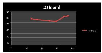
As observed from the graph the amount of CO in the exhaust increases at higher values of RH. This can be counted as a disadvantage of humidification technique, but as we can see that the increase is not too large and can be considered to be within the permissible limits.
