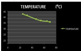
As we can observe in the graph, with increasing RH the temperature goes on decreasing which is in resemblance with the expected results.
