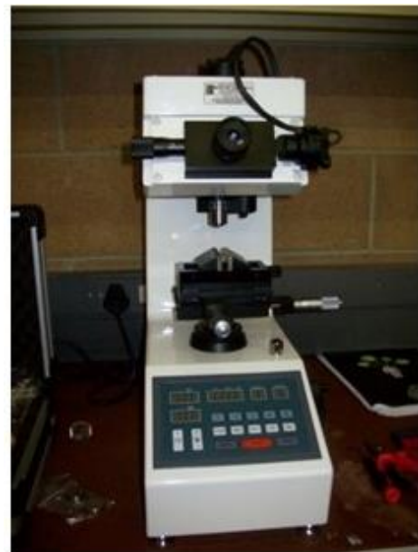
Figure 5 TIME HM-6 digital Micro-hardness testing machine
