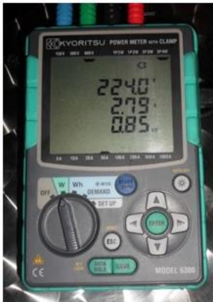
Figure 4. Three phase Kyoritsu power meter
