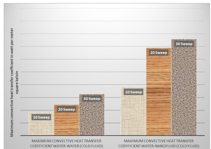
Figure 4: Graphical representation of Maximum Convective Heat Transfer coefficient of cold fluid for 10 sweeps, 20 sweep and 30 sweep
