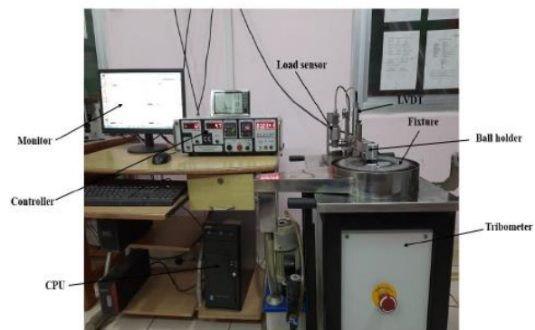
Fig. 3.5. Ball on disc tribometer
