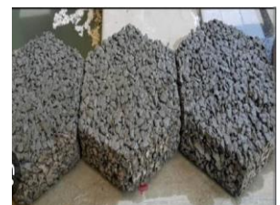
Figure 2: Hexagonal shape Paver blocks Figure 3: Previous Paver blocks
