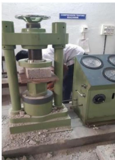
Figure 4: Compressive Strength test
